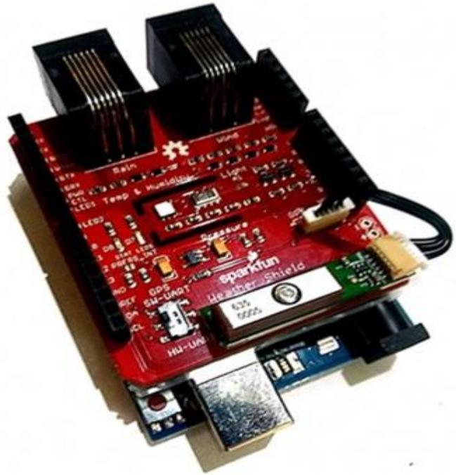
Fig. 5 Assemble Arduino, Sparkfun, and GPS.
