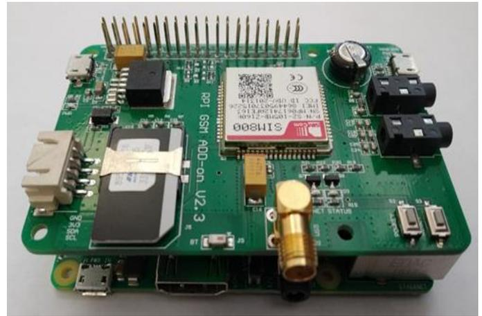
Figure 5. Raspberry PI with GSM ADD-ON.
