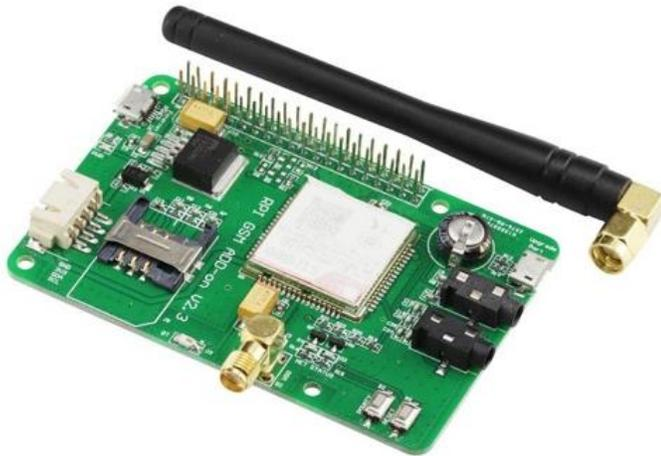
Figure 4. GSM ADD-ON v2.3. card
