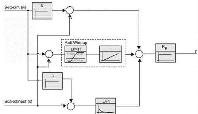
Fig. 10 Integration of PID parameters.
