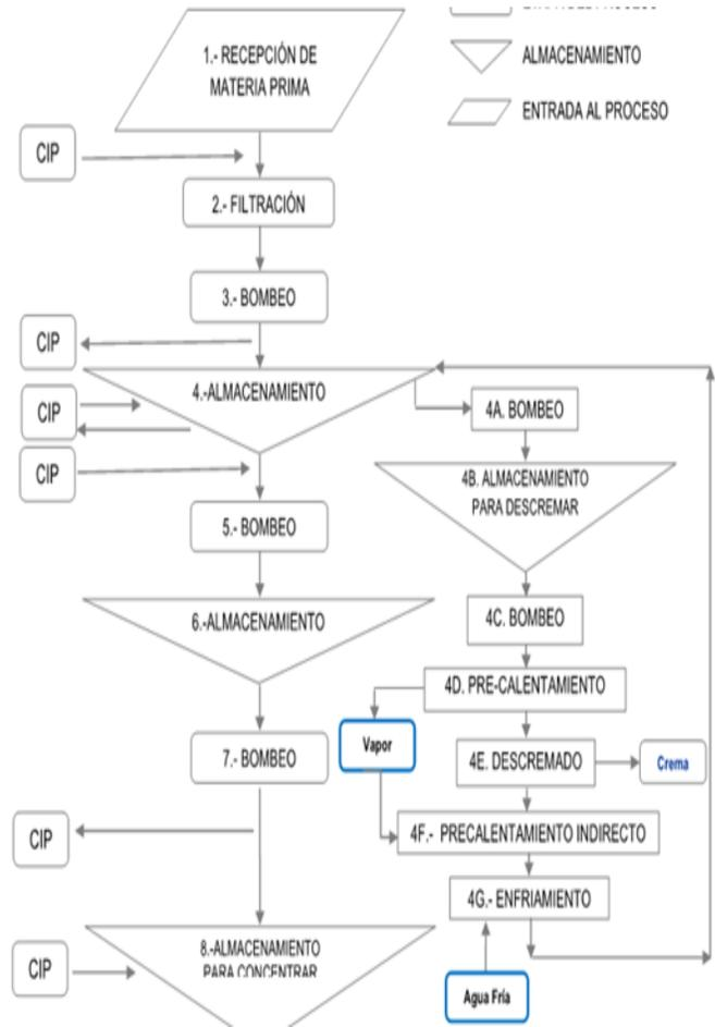
Fig. 2 Pasteurization system flow diagram.
