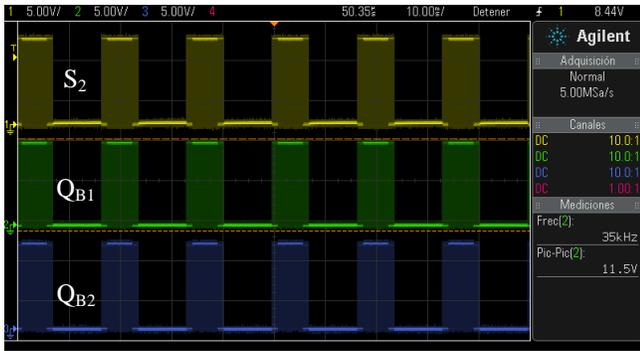
Fig. 6 SPWM triggering signals on leg B ( $S_2$ ,  $Q_{B1}$  and  $Q_{B2}$ )
