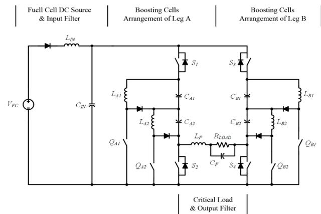
Fig. 1 Schematic diagram of the proposed Integrated DC-AC Back-up Fuel Cell Single-phase Converter.
