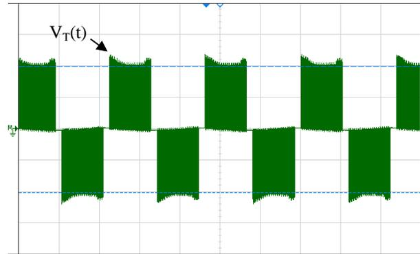
Fig. 8 Unfiltered output voltage from 5 VDC input voltage. Resolution: 5 V/div, 5 ms/div.
