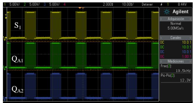
Fig. 5 SPWM triggering signals on leg A ( $S_1$ ,  $Q_{A1}$  and  $Q_{A2}$ )
