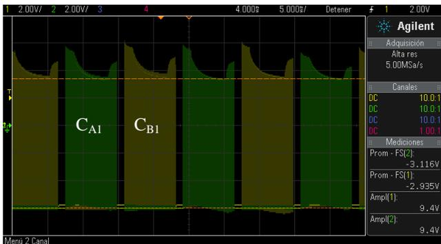
Fig. 7 Voltage measured respect to ground on  $C_{A1}$  and  $C_{B1}$
