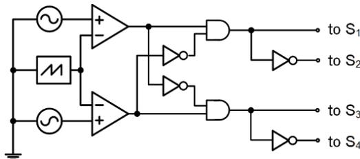
Fig. 3 Control logic to implement a modified unipolar SPWM scheme.
