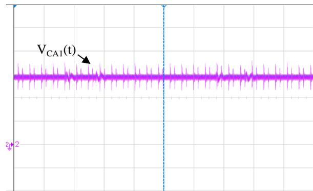
Fig. 9 Voltage on  $C_{A1}$ . Resolution: 2 V/div, 10 µs/div.
