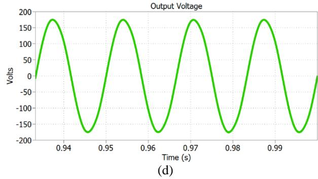
Fig. 4 Simulation results of the proposed IBFCSC; a) input current, b) voltage stored on  $C_{A1}$  &  $C_{A2}$ , c) pre-filtered output voltage, & d) 60 Hz sinusoidal output voltage.
