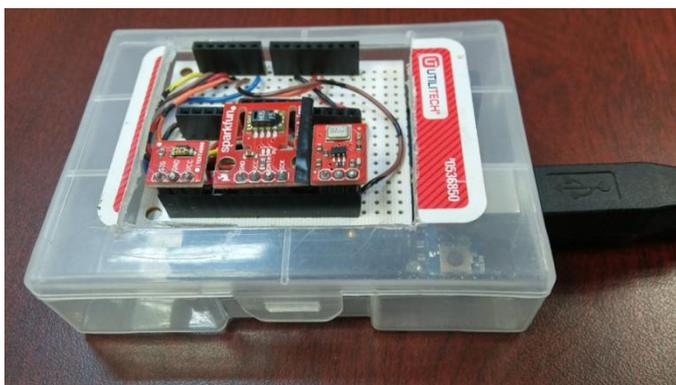
Fig. 4. Arduino framework for sensing application.
