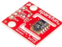
Fig. 1. SHT15 Temperature & Humidity Sensor.
