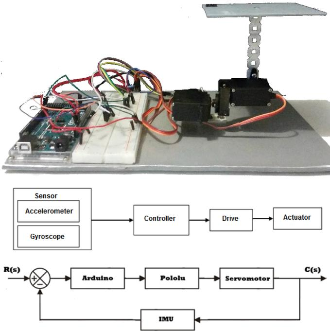
Figure 1. Platform prototype.
