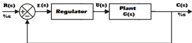
Figure 7. Diagram of System blocks.
