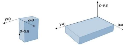
Figura 3. Accelerometer components.
