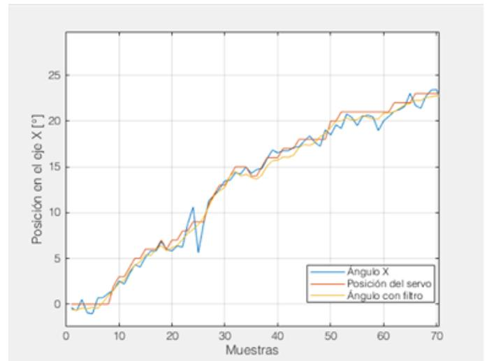
Figure 9. Actuator response in X-axis.
